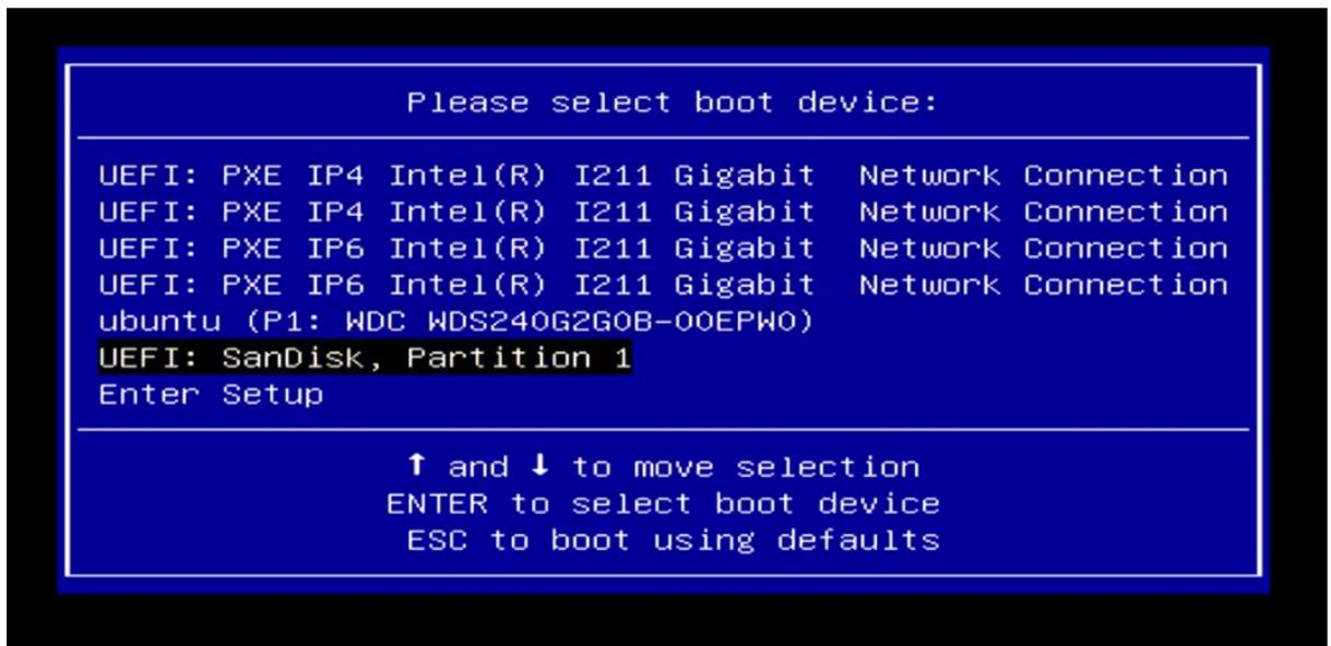
4. Now select the drive that is the USB device. The naming of this device differs between different USB stick vendors. The USB stick is not a device starting with IB... or P1... In the above case the USB stick is "SandDisk". Use the up/down arrow keys to select the device and press ENTER to boot.
