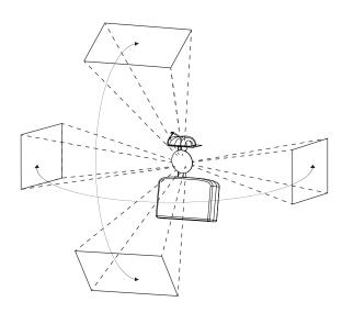
The Mirror Head is a modern high-tech mirror that is digitally operated and is used as an add-on feature for projectors. It can be set to move either rapidly or slowly to project pictures, videos and texts onto any imaginable surface.
